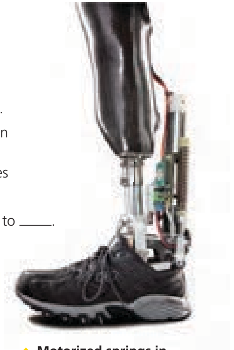
Motorized springs in a powered ankle push off like a real leg.
